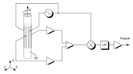
Fig. 3. Tubular piezoelectric angular rate sensor [3]
