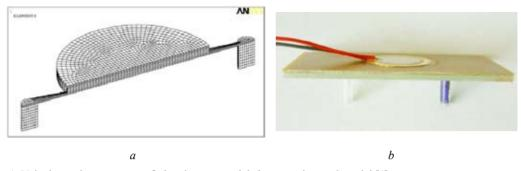
Fig. 1. Valveless micropump: a – finite element model; b – experimental model [1]
