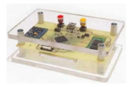
Fig. 5. Foot-mounted MEMS inertial measurement unit (IMU) [5]
