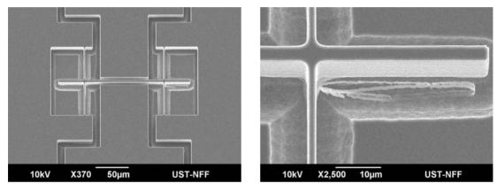
Fig. 2. SEM images of micromechanical resonator [2]
