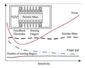
Fig. 4. Accelerometer sensitivity vs. noise trade-off analysis
