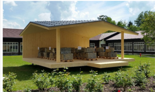
Figure 6: Outdoor test stand with a permanent loading at the Bern University of Applied Sciences.
