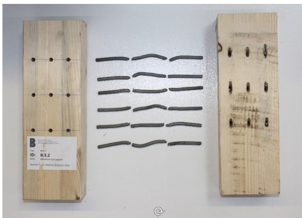
Fig. 11. Cyclic tested and opened connection with broken dowels due to low-cycle fatigue (specimen B.3.2).
