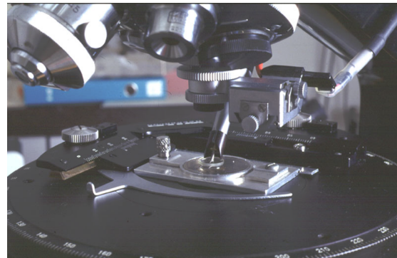
Fig. 3: Photograph showing the diamond micro-drill mounted on a conventional optical petrographic microscope.
