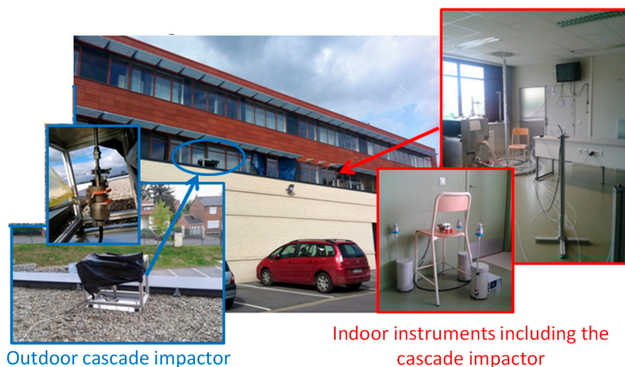
Figure 2. Pictures of the cascade impactors installed either inside the investigated classrooms (red) or outdoors (blue) during the field campaign.
