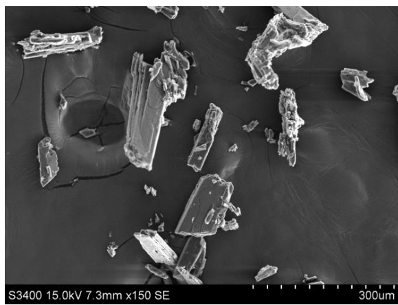
(c) Load 7: \text{KHCO}_3 crystal sampled at 60°C
