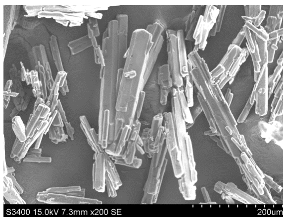
(b) Load 5: crystal sampled at 24.8°C
