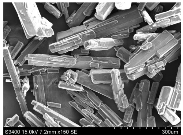
(b) Load 7: AMP bicarbonate and \text{KHCO}_3 crystals sampled at 49°C
