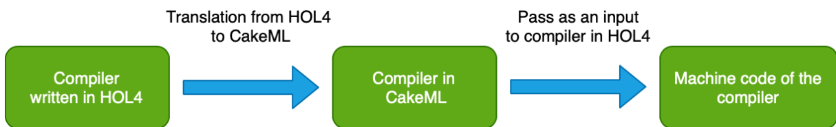
Fig. 3. Sequence of transformations for generation of a formally-verified machine code using the CakeML compiler and HOL4 proofs.
