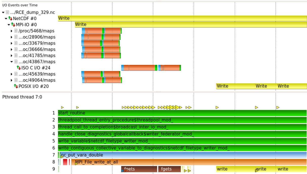
Figure 5.15: The I/O timeline (top) shows individual I/O operations of Pthread thread 7:0 (Thread 7 of the I/O server process Rank 0) on specific files. The tree view on the right hand side reflects the recorded hierarchical relations between files. The process summary (bottom) depicts the corresponding call stack and illustrates interactions of the individual layers of the I/O software stack. For instance, the NetCDF routine nc_put_vara_double (blue bar, call stack level 7) internally calls the MPI I/O routine MPI_File_write_at_all (orange bar, call stack level 8) which utilizes POSIX I/O functions (brown and yellow bars, call stack level 9).
