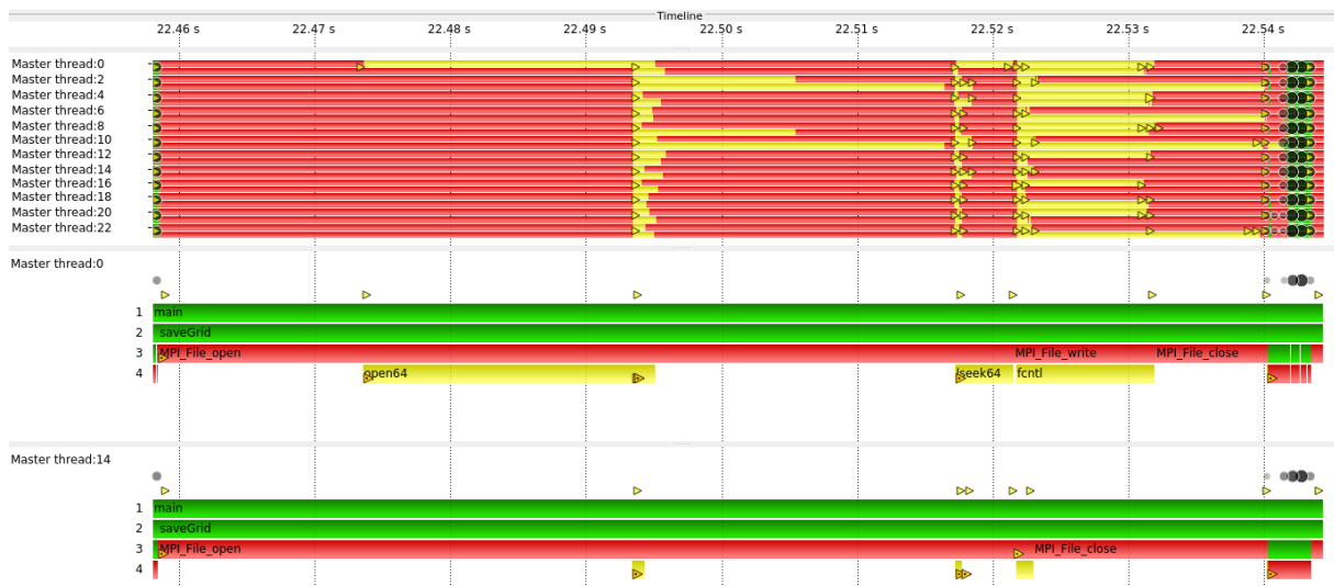
Figure 5.7: This figure illustrates the application behavior during the time interval of writing a snapshot to the result file. The upper chart gives an overview of current activities across all processes. Red bars represent MPI routines, yellow bars indicate I/O operations, and green bars reflect user functions. The middle and lower chart depict the sequence of function calls for MPI Rank 0 ( Master thread:0 , top) and 14 ( Master thread:14 , bottom). The saveGrid routine (green bar, call stack level 2) generates a snapshot. This routine utilizes MPI I/O to transfer data to the result file, e.g., MPI_File_open , MPI_File_write , and MPI_File_close (red bars, call stack level 3). The call stack visualization reveals internal I/O library calls within the MPI I/O routines. For instance, the middle chart depicting Master thread:0 shows that MPI_File_open calls the POSIX I/O routines open64 and lseek64 (yellow bars, call stack level 4). Additionally, the upper chart indicates an imbalance in the execution time of open64 calls across all processes (variable length of the yellow bars).
