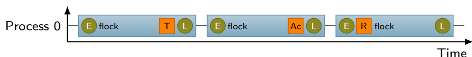
Figure 3.15: Example of a sequence of file locking operations and their corresponding I/O events.
