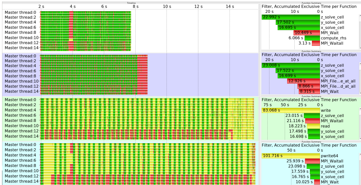
Figure 5.8: This figure compares the I/O modes in NAS BT-IO (problem size Class A , 16 processes). It contrasts all four modes from top to bottom: epio (white background), full (purple background), fortran (green background), and simple (azure background).
