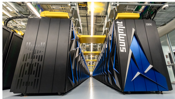
(b) The Summit supercomputer (IBM system equipped with IBM POWER9 processors and NVIDIA Volta V100 GPUs, theoretical peak performance of 200 petaflops). (Photo by OLCF at ORNL / CC BY 2.0)
