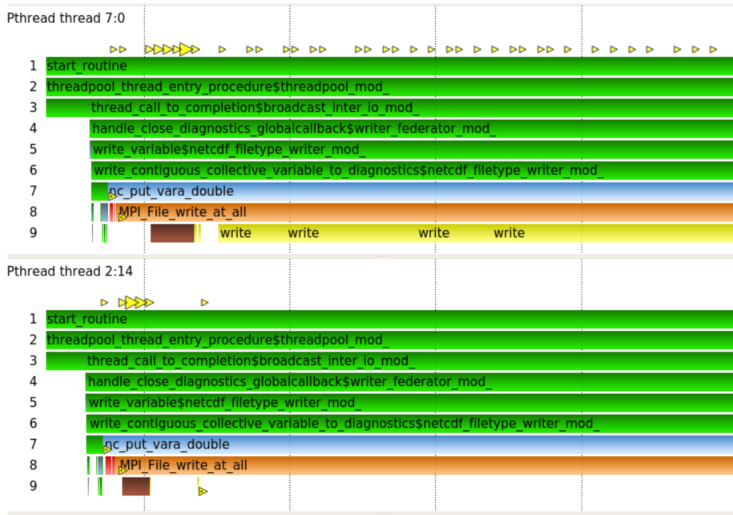
Figure 5.16: This figure compares the call stacks of two different MONC I/O server processes. Both servers show an identical call stack except level 9. Only the I/O server process shown in the top chart issues calls to the POSIX I/O write routine (yellow bars).
