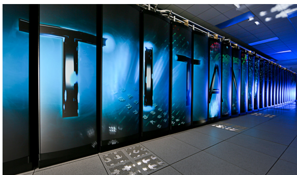
(a) The Titan supercomputer (Cray XK7 system equipped with AMD Opteron processors and NVIDIA Kepler K20X GPUs, theoretical peak performance of 27 petaflops). (Taken from [31])
