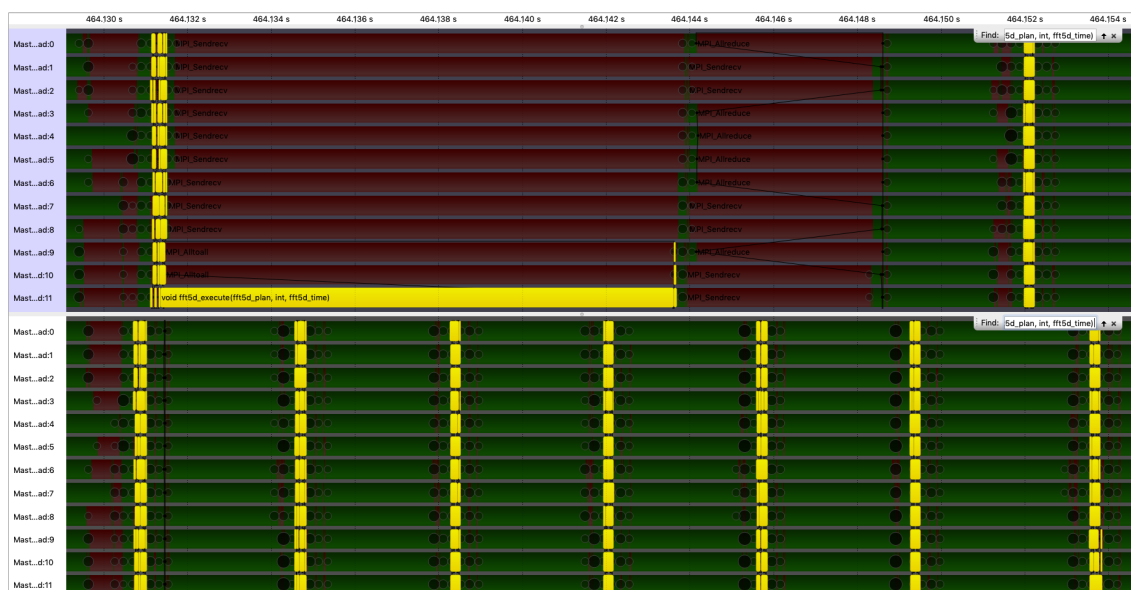
Figure 5.22: Event log visualization of GROMACS Job 12154380, Job Step 2 . The upper graph (blue background) shows an event sequence of the GROMACS run with disabled load balancing. The lower graph (white background) illustrates the corresponding event sequence of a run with enabled load balancing. The event sequences depict GROMACS functions (green) and MPI communication (red). Invocations of the function ffs5d_execute are highlighted in yellow. As the lower graph shows, improved load balancing results in a considerable reduction of the time required to execute an iteration.
