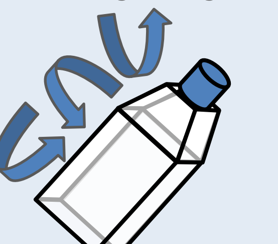
Figure 9: This is a graphic representing a tissue culture flask that will be used to culture cells in an simulated microgravity environment. The flask rotates continuously on an x, y, and z plane simultaneously while also moving in a figure-8 motion.
