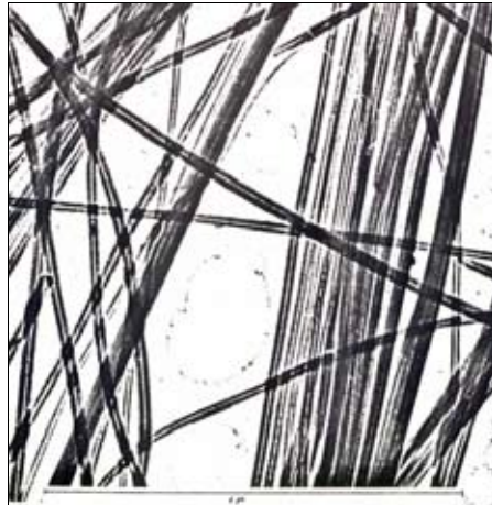
Fig. 1. Asbestos fibers under the microscope. The fibers that are visible to the naked eye are composed of hundreds of thousands mono-fibers called fibrils in close packed parallel arrangement
