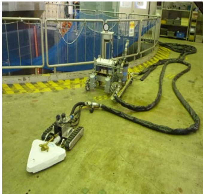
Figure 54 - The Raccoon Floor decontamination (TEPCO 2016)
