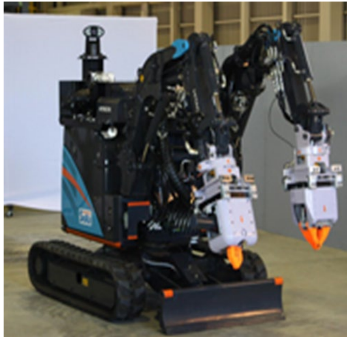
Figure 55 - Debris Removal Robot (ASTACO-SoRa) (TEPCO 2016)
