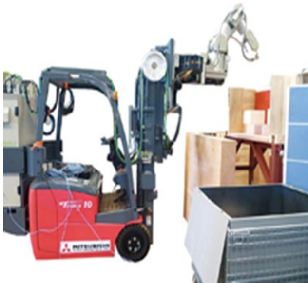
Figure 48 - Used to Remove Shielding Blocks (TEPCO 2016)
