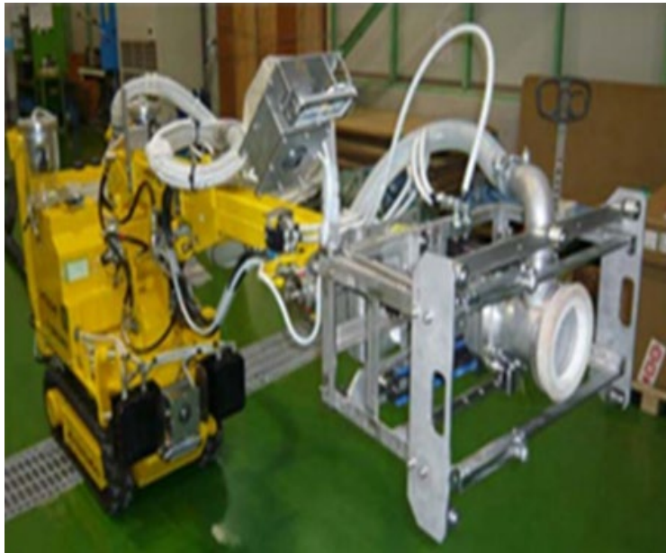
Figure 49 - High Pressure Decontamination Robot (TEPCO 2016)
