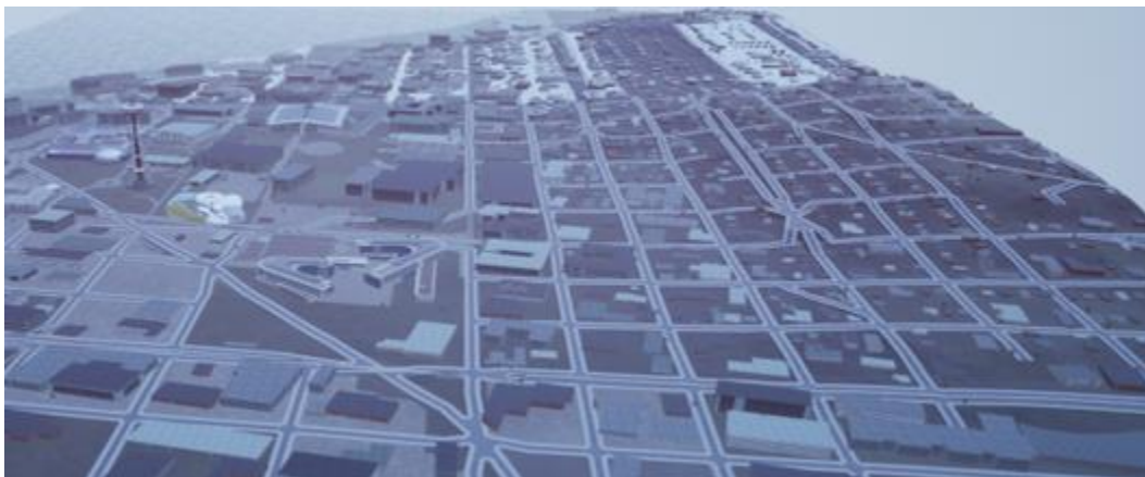
Figure 42. Depiction of multiple LODs within the visual scene. The lower LOD can be observed in the top section of the figure when compared to the above figure. Scene rendered in UE4.
