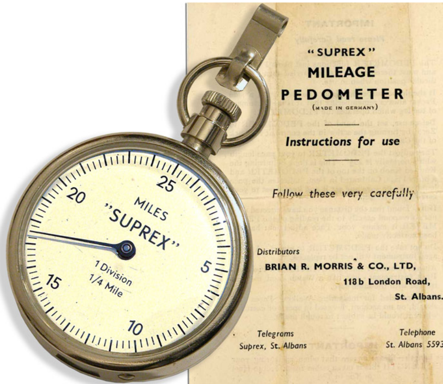
Figure 1.3: Example of a common early pedometer. The Suprex was a German pedometer manufactured in the 1970s and functioned with a mechanical lever that activated internal gearing, in turn increasing the displayed mileage count.
