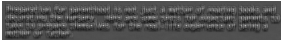
Figure 1.8: The MSF image for the NCC example. Notice how bright spots occur at the locations corresponding to the center of all letters that resemble an 'e' in the original image.
