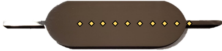
Figure 12: Cantor alloy specimen used for microhardness experiments. Indents denoted by colored diamonds (not to scale).
