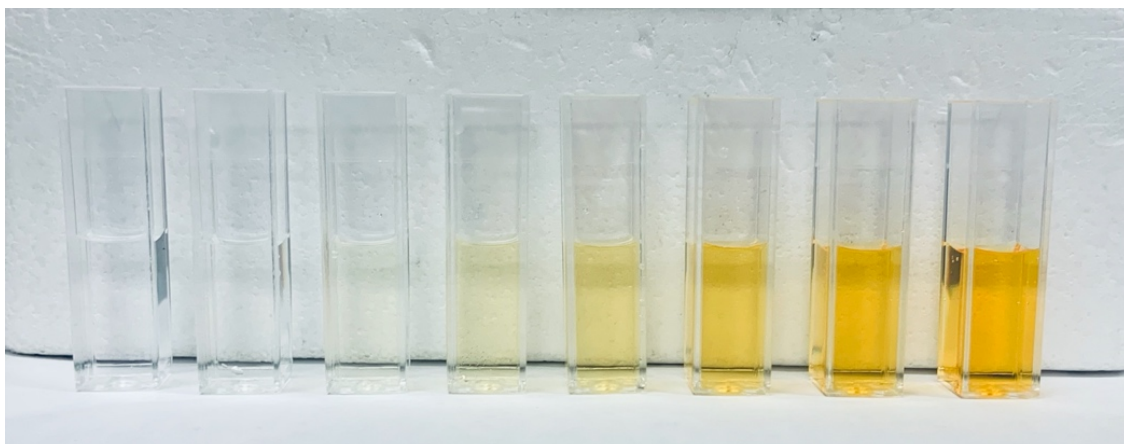
Figure A-3. Spectrophotometric measurement of H 2 O 2 standards using titanium oxysulfate method – concentration increases left to right.
