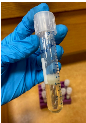
Figure 4: Image of K. xylinus culture grown in 15 mL tubes. The top opaque layer indicates a healthy layer of BC forming on top.
