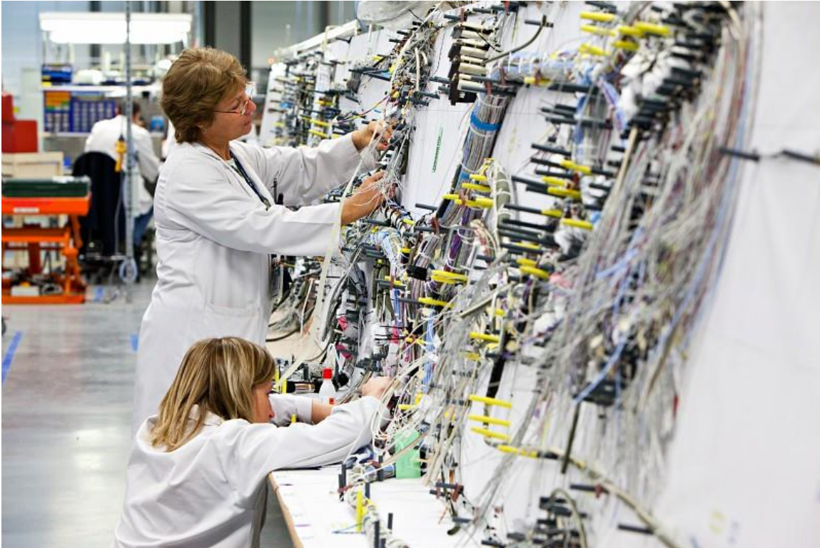
Figure 3.1: SAFRAN team members assembling airplane wire harness assemblies for a military aircraft. The complex shape and number of critical components make this a heavily manual process. There are many opportunities for mistakes during assembly.
