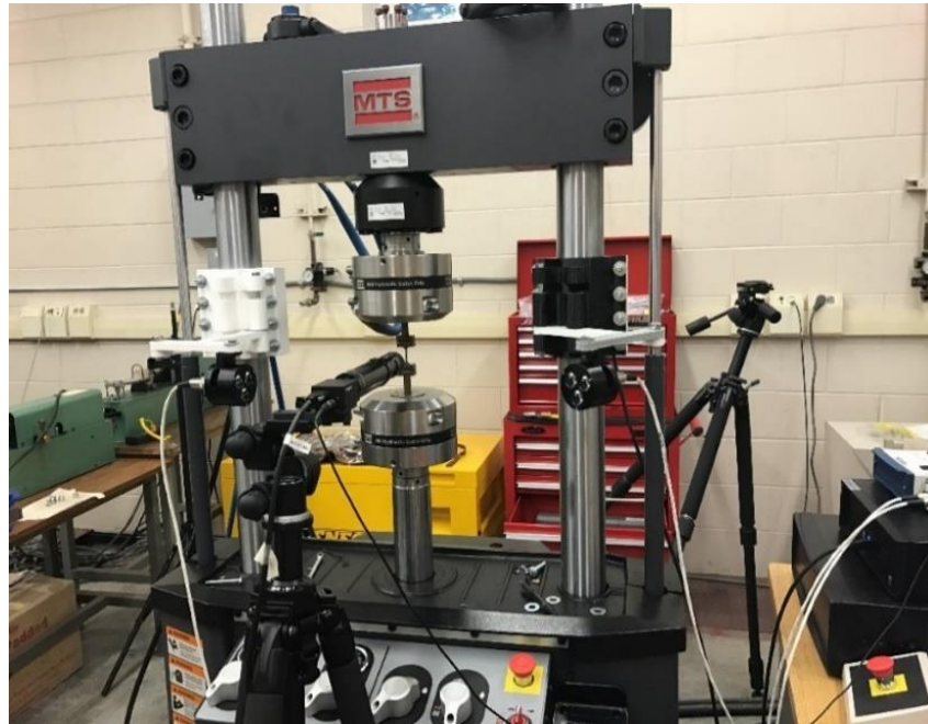
Figure 9. Camera and light setup to use DIC for a tensile mechanical
