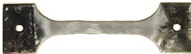
Figure 16. Surface of the sample post-mortem revealing out of plane deformation causing the images to be out of focus for HRDIC purposes.
