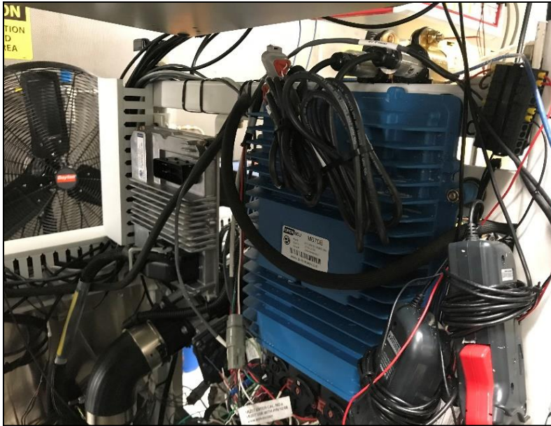
Figure II-2: Pi Innovo OpenECU M670B installed in the test cell.
