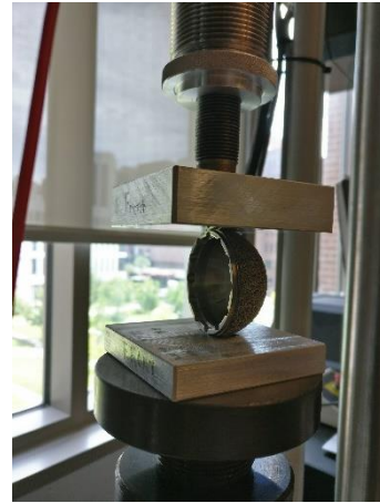
Figure 2: (a) Schematic showing the test method setup, with the dotted arcs representing the grooves cut into the plates to hold each device in place (b) Test setup with a device held in place by the plates
