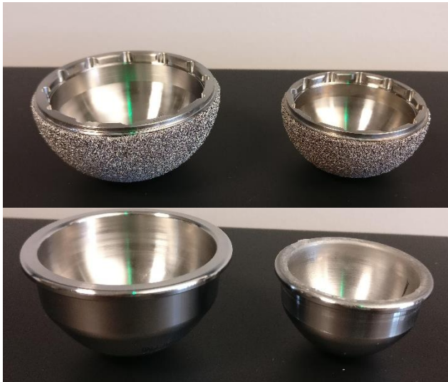
Figure 1: (a) Acetabular shells, 62 mm and 50 mm respectively (b) Acetabular shells, size 62/50 and 50/38 respectively. These are the CoCrMo HC liners, but the LC and SS liners were identical in design
