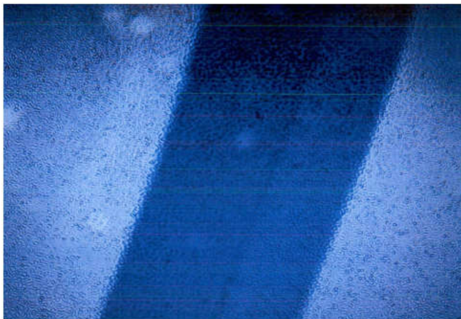
Figure A-10: Image at 4x Magnification for Cellular Response to Polymerized MPC-S with L929 Cells (dots) and Sample Placement Area (dark outline) Visible
