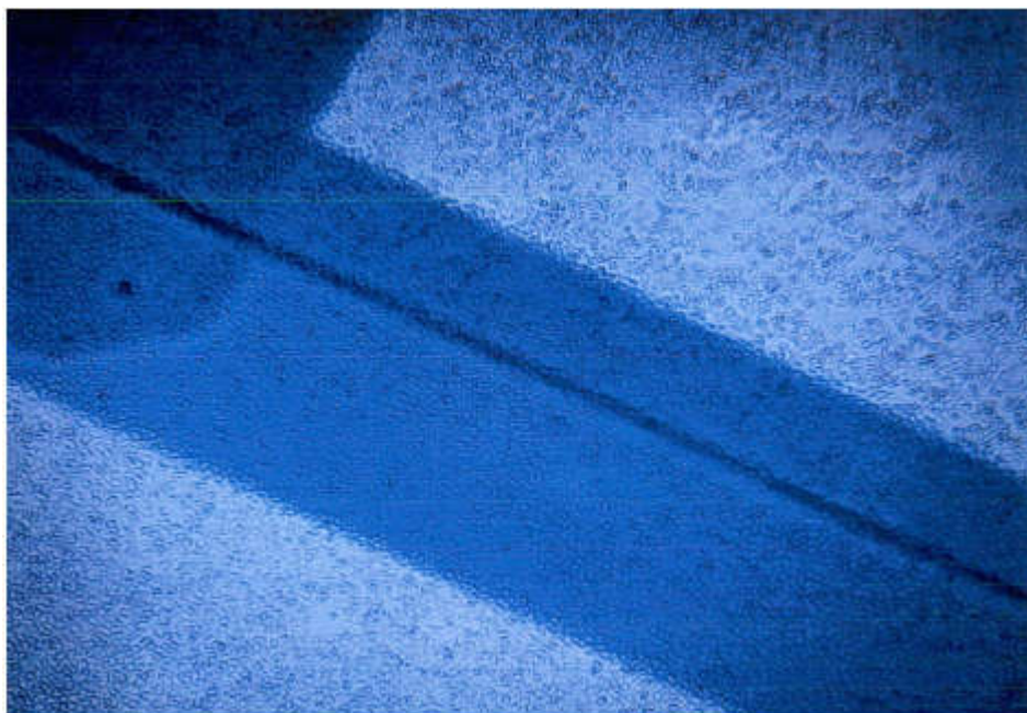
Figure A-11: Image at 4x Magnification for Cellular Response to Polymerized BCA with L929 Cells (dots) and Sample Placement Area (dark outline) Visible
