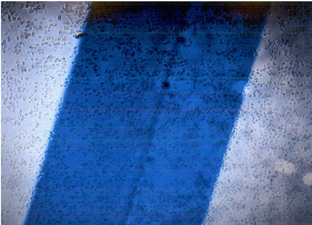
Figure 5-18: Cytocompatibility Results Image at 4x Magnification for Cy90-G40C60T10 with L929 Cells (dots) and Sample Placement Area (dark outline) Visible
