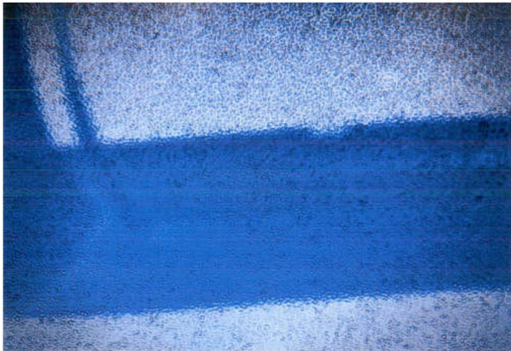
Figure A-6: Image at 4x Magnification for Cellular Response to Polymerized Cy90-G10C90T10 with L929 Cells (dots) and Sample Placement Area (dark outline) Visible
