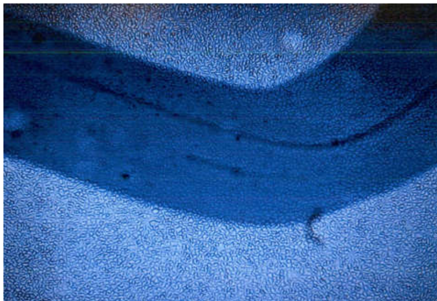
Figure A-1: Image at 4x Magnification for Cellular Response to Polymerized Cy96-G10C90L4 with L929 Cells (dots) and Sample Placement Area (dark outline) Visible
