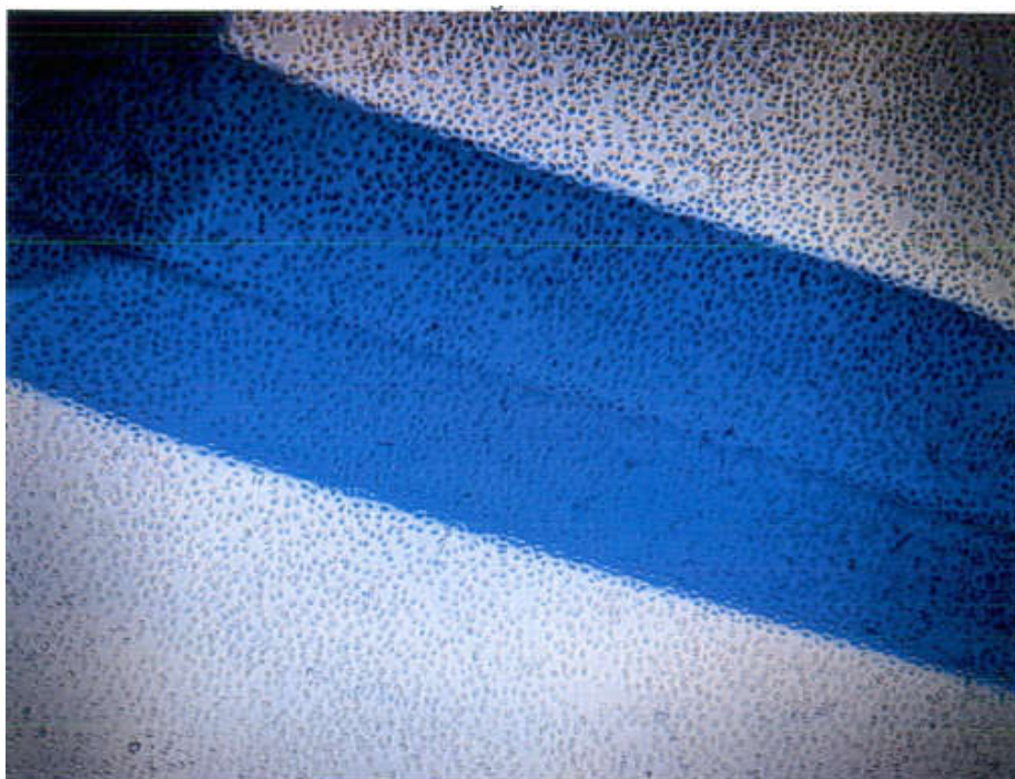
Figure A-9: Image at 4x Magnification for Cellular Response to Polymerized EEC with L929 Cells (dots) and Sample Placement Area (dark outline) Visible
