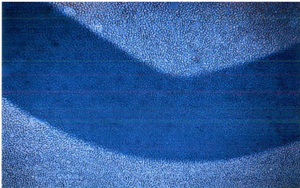
Figure A-4: Image at 4x Magnification for Cellular Response to Polymerized Cy90-G40C60L10 with L929 Cells (dots) and Sample Placement Area (dark outline) Visible
