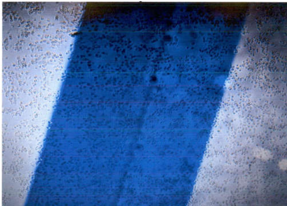
Figure A-8: Image at 4x Magnification for Cellular Response to Polymerized Cy90-G40C60T10 with L929 Cells (dots) and Sample Placement Area (dark outline) Visible
