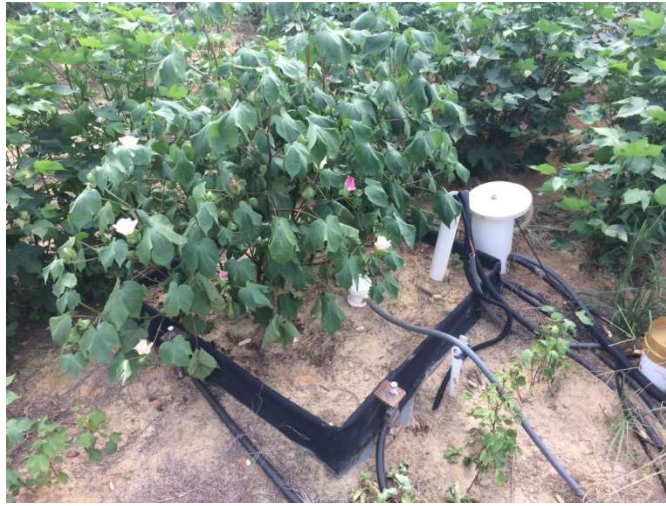
Figure 1.5. Weighing Lysimeter Planted with Cotton
