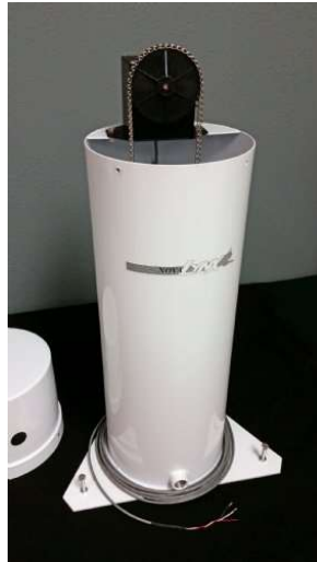
Figure 3.5. NovaLynx 255-100 Analog Output Evaporation Gauge (NovaLynx Corporation, 2016)
