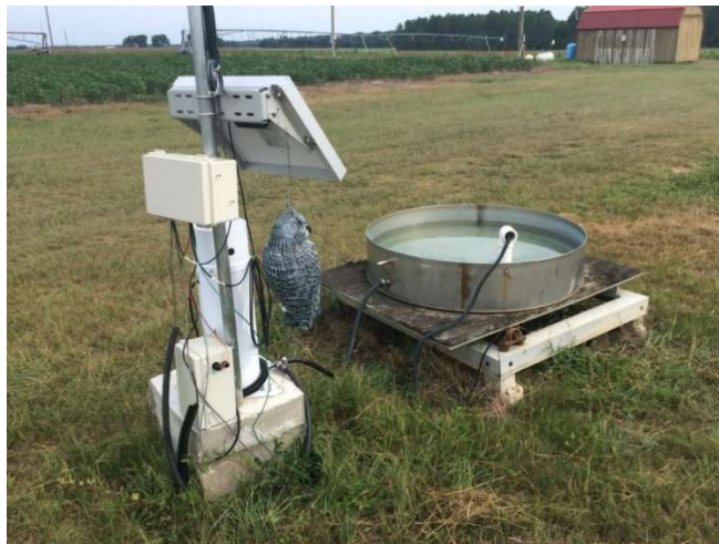
Figure 3.4. Pan Siting of Class A Evaporation Pan
