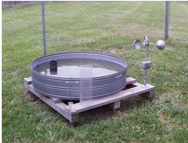
Figure 3.2. Class A Evaporation Pan Surrounded by Wire Enclosure
