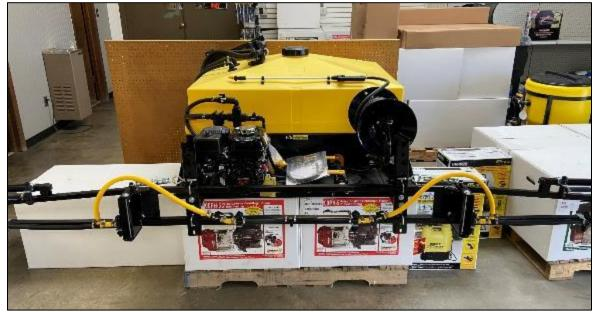
**Figure 16.** This is another slide-in spray unit set up with a 100-gallon tank. This option is equipped with a 30-foot boom and a hand-gun sprayer.
