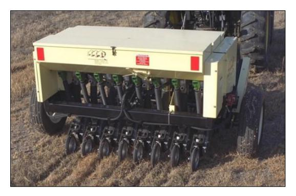
**Figure 22**. A Truax FLEXII no-till rangeland drill. There are eight drill rows on this planter, but they range from 6-22 rows depending on the unit purchased. This drill was used for the CSU revegetation plots at DEN.
