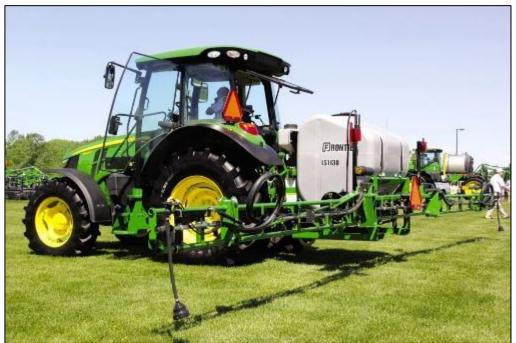
**Figure 14.** John Deere LS1130 sprayer equipped with a 300-gallon tank and a 30-foot boom (Garvey 2017).
