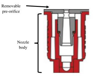
**Figure E3.** TeeJet XR 11003 nozzle body. The grey colored part of the nozzle is the pre-orifice that can be pulled out of the nozzle body. To clean the nozzle, use a soft brush to clean the tip of the nozzle body and pre-orifice.
