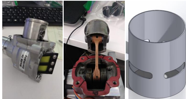
Figure 47: 3w-28i Engine Specs [57], disassembled 3w-28i engine, Piston and connecting rod exposed, and SOLIDWORKS model of the cylinder with three intake ports and an exhaust port
