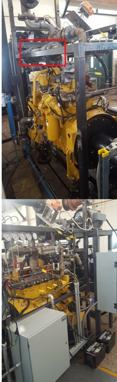
Figure 3.4: Experimental setup for the Caterpillar G3304 engine operating with dedicated EGR and upgraded measurement and control capabilities. The EGR mixer is shown in the red box.
