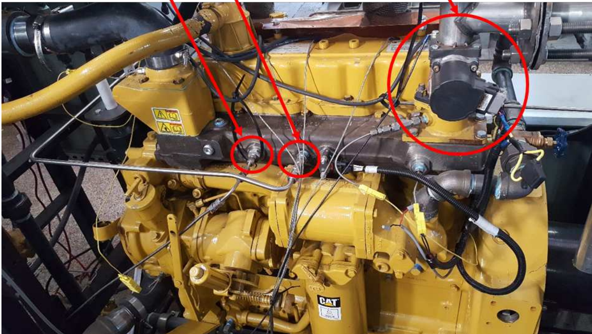
Figure A.16: 'Cold side' of the G3304 engine. The delivery of additional fuel to the dedicated cylinder via port fuel injection is highlighted. The intake manifold composition measurement and engine speed control are also highlighted.
