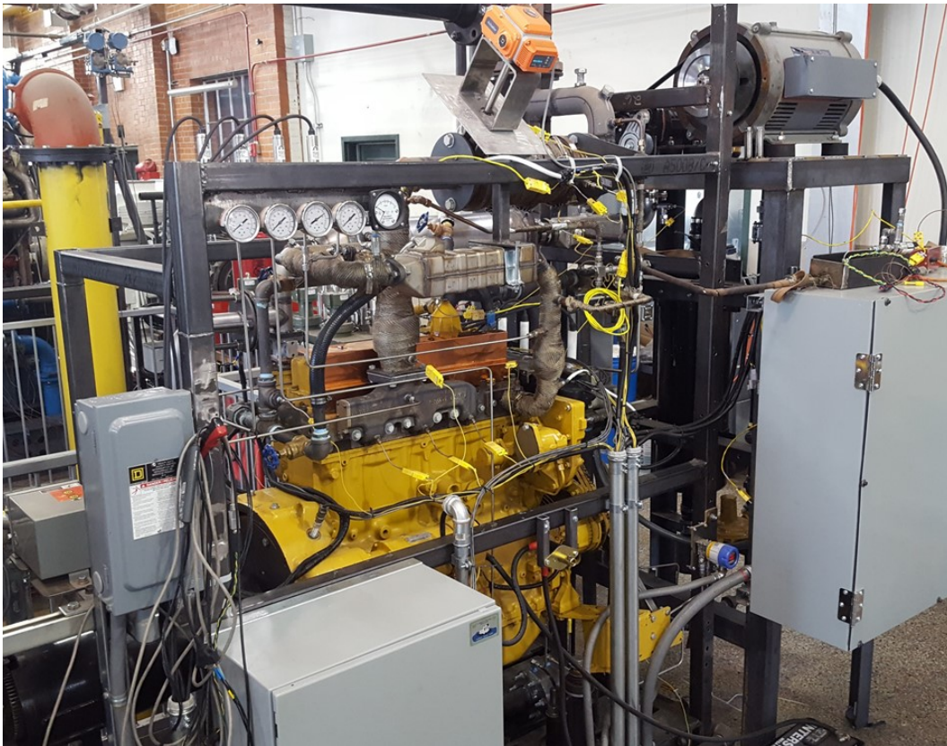
Figure 4.2: Experimental engine test cell used for this work.
