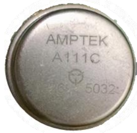
Figure 3.1. A photograph of the Amptek A111 chip, with metal housing.
