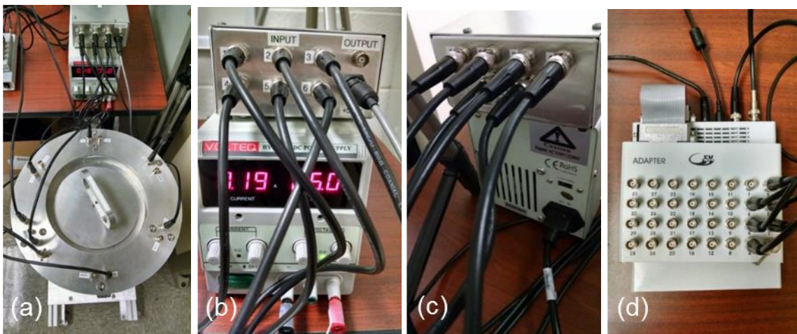
Figure 6.2. The BCS HLNCC showing (a) the six detector bank outputs; (b) the BCS HLNCC-specific conversion box containing electronics to shape and amplify the output signals, resting on the external power supply used for the +5 V; (c) the output signal cables of the conversion box; and (d) PTR-32.
