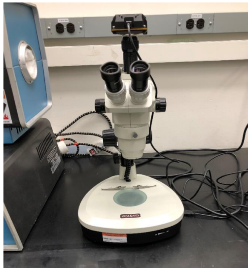
Figure 3-11 Omana OM4424 Dual-Power 20X / 40X Stereo microscope used to inspect samples as they were being polished.
