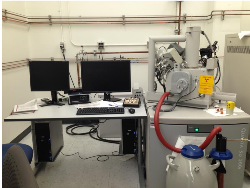
Figure 3-20 FEI Quanta Dual-beam FIB/SEM that is located in the LAMDA facility in ORNL.
