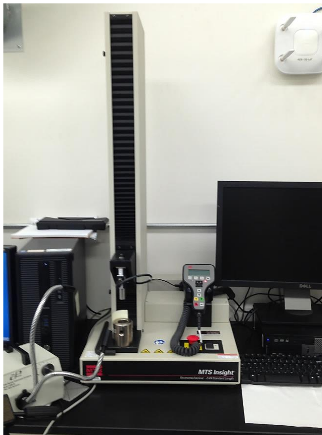
Figure 3-32 MTS tensile screw-driven machine (model Insight 2-52) system used for the 3-point bend test experiments.
