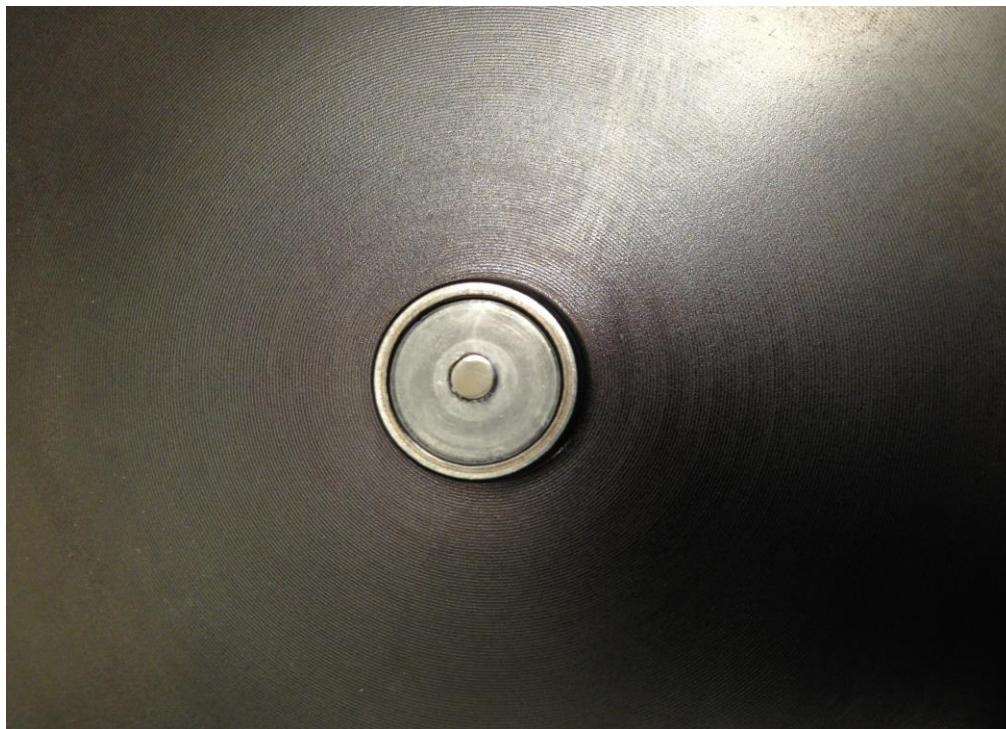
Figure 3-10 Cu based BMG 3 mm disc specimen secured in the top holder device.
