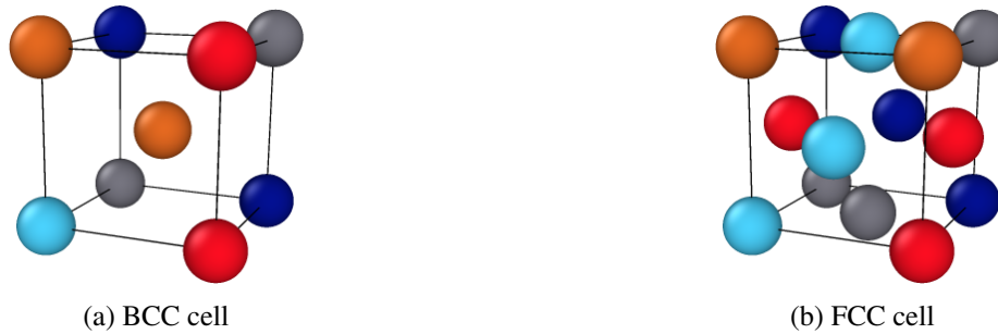
Figure 4.2: Example of body-centered cubic, (BCC), (a) and face-centered cubic, (FCC), (b) unit cells without additive noise or sparsity. Notice there is an essential topological difference between the two structures: The body-centered cubic structure has one atom at its center, whereas the face-centered cubic is hollow in its center, but has one atom in the middle of each of its faces.
