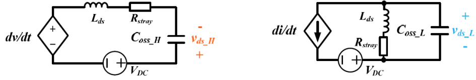
Fig. 2-6. Equivalent circuits of turn-on and turn-off transients [29].
