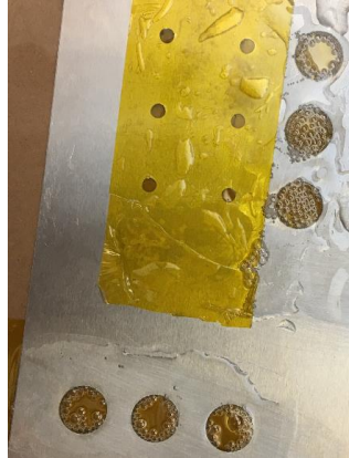
Fig. 7-17. Busbar under vacuuming inside vacuum chamber.
