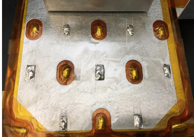
Fig. 7-19. Soldering joints of capacitors on aluminum busbar.
