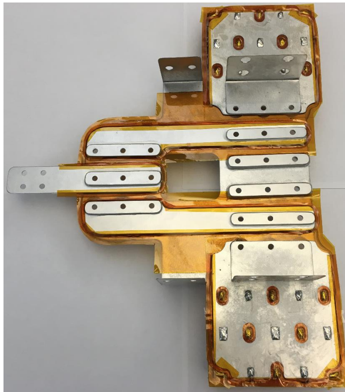
Fig. 7-20. Bottom view of fabricated busbar for a 500 kVA 3L-ANPC converter phase leg.
