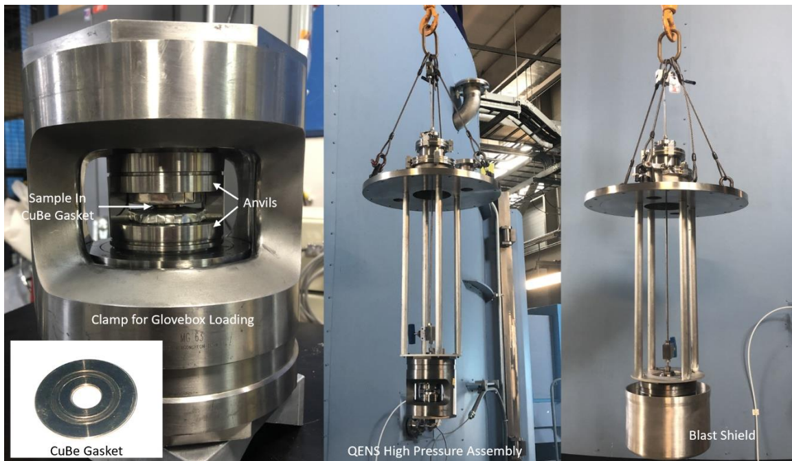
Figure 7: Paris-Edinburgh cell with a stand assembly for QENS experiments at BASIS. One of the CuBe gasket halves is shown.
