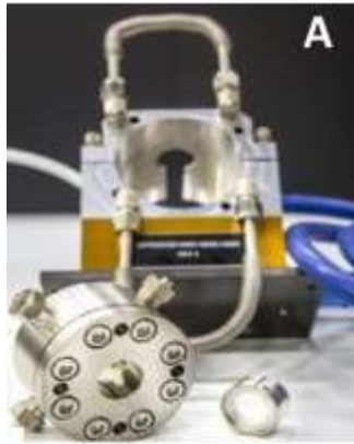
Figure 3.6: A). The assembled enhanced angle pressure cell with its holder. 2 The pressure cell has two sapphire windows and a spacer (seen next to the cell) that modulated the thickness of sample. B). Pressure profile of water filled in the pressure cell during heating phase from 25 °C to 180 °C and cooling phase of 180 °C to 25 °C
