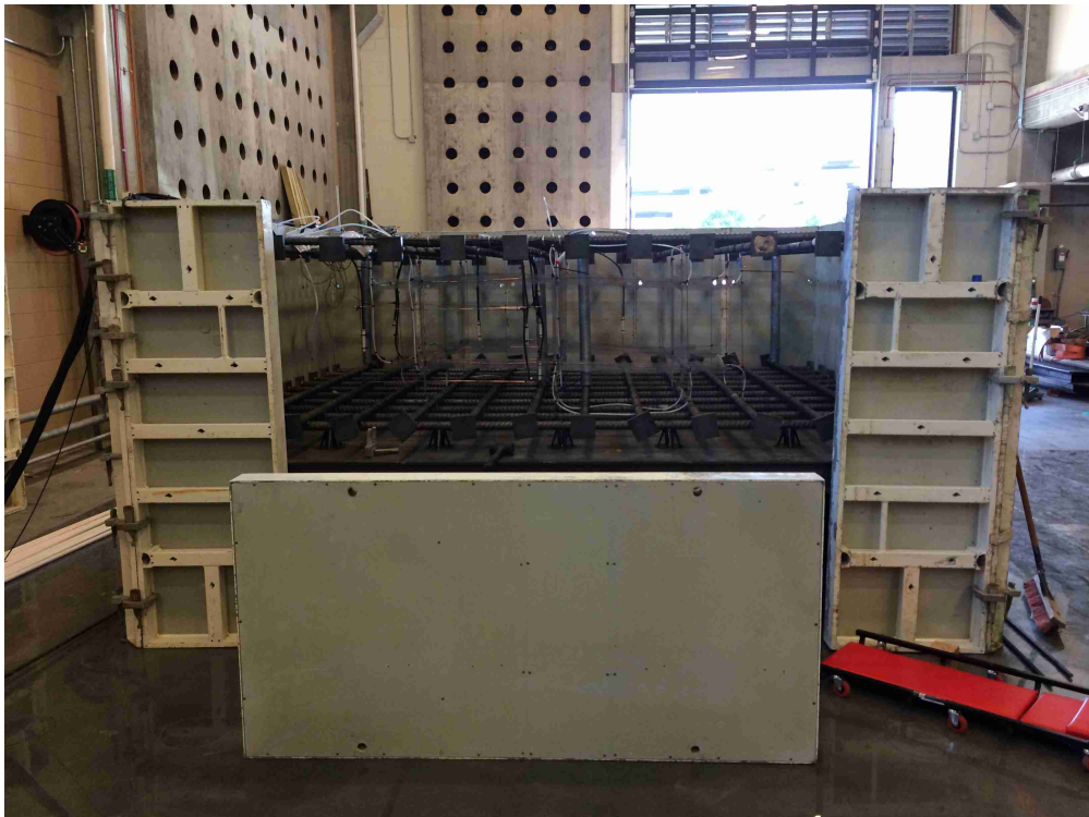
Figure A.6: Partially assembled side formwork system
