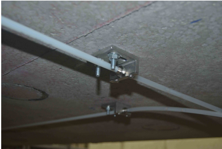
Figure A.10: SOFO deformation sensor attached to bottom surface of concrete specimen
