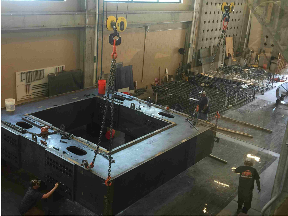
Figure A.8: Assembled steel confinement frame
