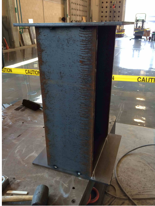
Figure A.3: Unpainted assembled steel support
