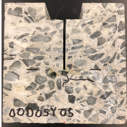
Figure 3.9: Evidence of horizontal crack propagation in the 00D1Y specimen with crack outlined below notch tip.
