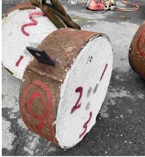
Figure 3.4: Photo of concrete inside confinement prior to cutting.
