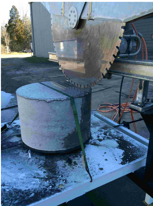
(a) Confined cylinder cutting
