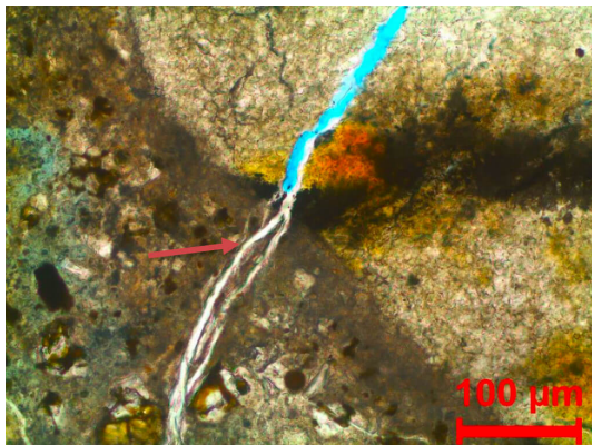
(c) Crack in aggregate and cement
