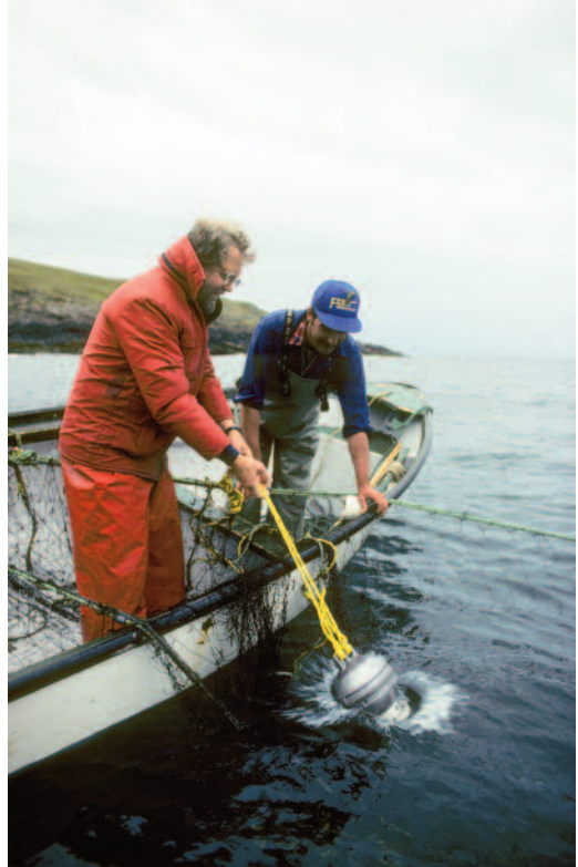
FIGURE 2. Jon Lien attaches whale alarma to a cod net.
