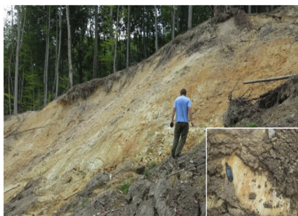
FIGURE 6. Crown of the rockslide with the sliding surface in the central part of the rockslide (detail of sliding surface in mylonites)
