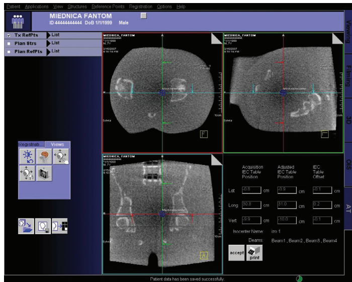
Fig. 1. Main screen of the Adaptive Targeting software – Siemens Coherence Therapist Workspace. In the application, three views are presented to the user: the coronal, the sagittal and the frontal one. In the bottom right corner, the results of registration are provided. The images obtained with MVision are presented
