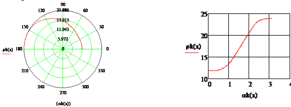
Figure 5 – Estimated cam profile and its radii of curvature at the pusher lift section
