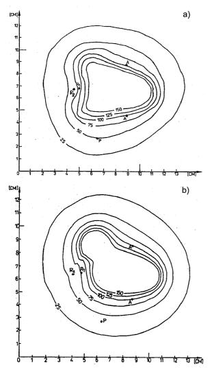
Dose distribution in XY plane: (a) from a stationary unit, (b) from a mobile unit.
