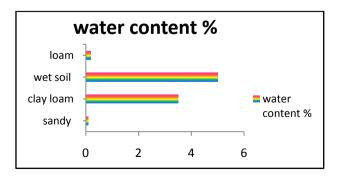
Figure 4: Graph representation of soil testing results
