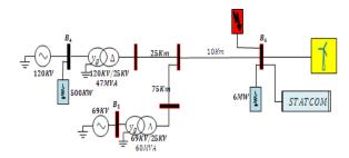
**Figure 3:** Modelling Wind farm with STATCOM[2]
