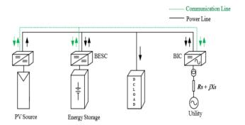
Figure 3: Single line diagram of a DC microgrid connected to the utility grid [14]
