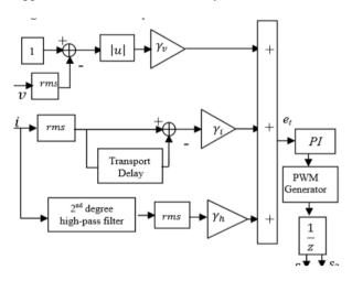
Figure 4: The Tri-loop dynamic error driven controlled PWM layout [23]
