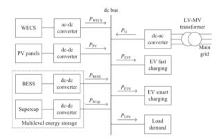
Figure 1: Layout of DC Microgrid [3]
