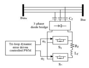
Figure 5: The MPFC layout [24]
