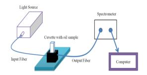
**Figure 2:** Experimental setup for UV-Vis Spectroscopy [16].
