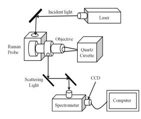
Figure 7: Schematic of CLRS Experimental Setup [25].
