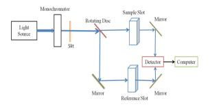
Figure 1: Block diagram of double beam spectrometer [14]
