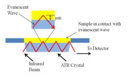
Figure 4: Principle of ATR technique [21]
