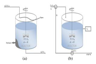
Figure 2: Non-linear CSTR: (a) Real system; (b) Model system [2]
