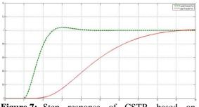
Figure 7: Step response of CSTR based on Adaptive controller when  $\gamma = 0.5$
