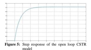
Figure 5 shows the open loop response of the nonideal CSTR where x-axis defines the time and yaxis defines the effluent concentration.
