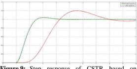
**Figure 9:** Step response of CSTR based on adaptive controller when  $\gamma = 1.5$
