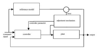
Figure 3: Model Reference Adaptive Controller
