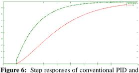
Igure 6: Step responses of conventional PID and IMC based PID controller
