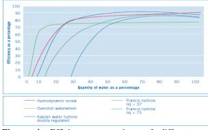
Figure 4: Efficiency comparison of different turbine types [15]
