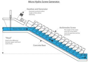
Figure 3: Basic model of Archimedes Screw Turbine [16]
