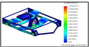
Figure 4: Von Mises Stress
