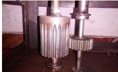
Figure 2: Gears mounted of different face widths 3. Automatic Lawn Mower Models
