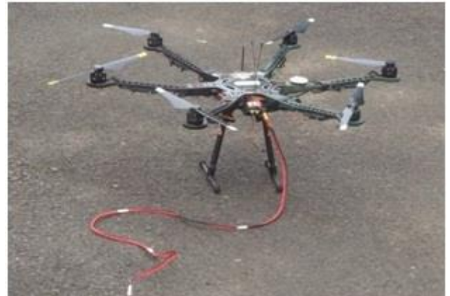
Fig. 9 Experimental set up of assembled hexacopter with tethering system
