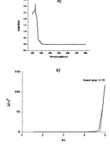
Figure 3: a) Absorption spectra b) tauc plot of ZnO nano particle using conventional method.
