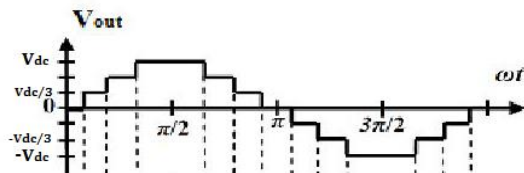
Fig.2.Output Waveform of 7 level Inverter
