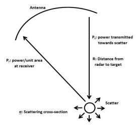
Figure1: Concept of radar equation.
