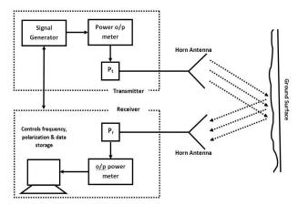
Figure2: Block diagram of active microwave sensor.
