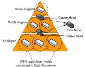
Figure5: Regionalized WSN architecture for landslides [32]
