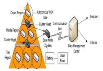
Figure11: Early Warning system for landslide in Mauritius.
