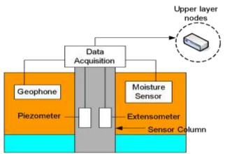
Figure4: WSN deployment with sensor column [32]
