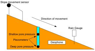
Figure3: Placement of landslide monitoring sensors [31]
