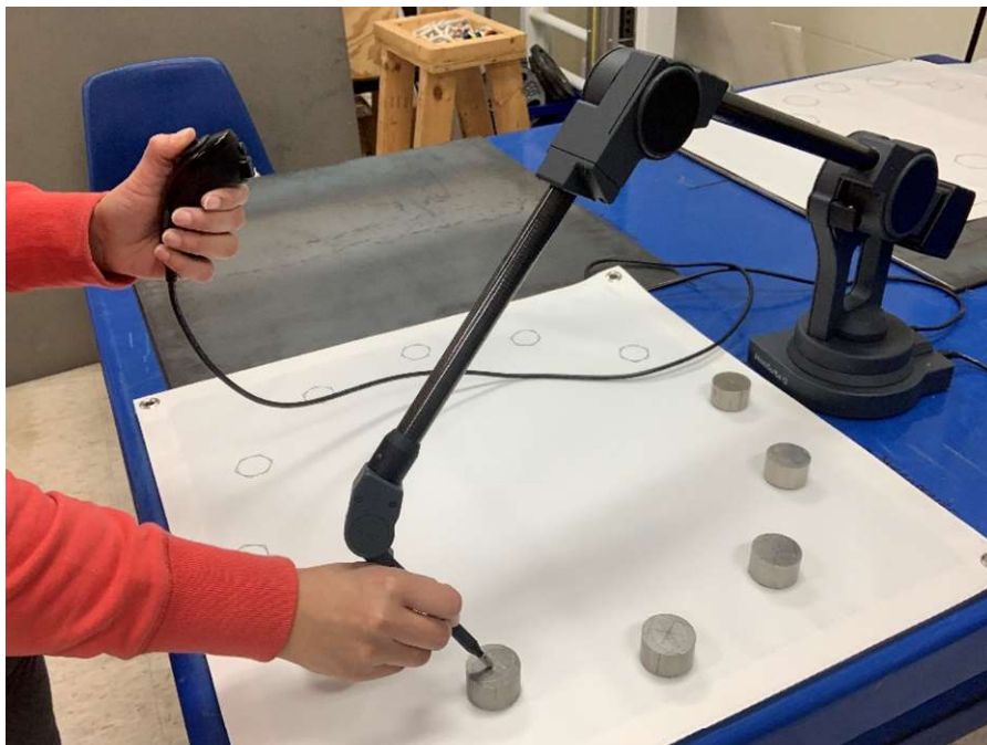
Figure 3-5: Digitizer used to capture center of target objects
