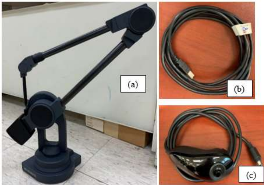
Figure 3-4: Microscribe Digitizer system : (a) Articulating arm unit (b) USB Cable (c) Input device
